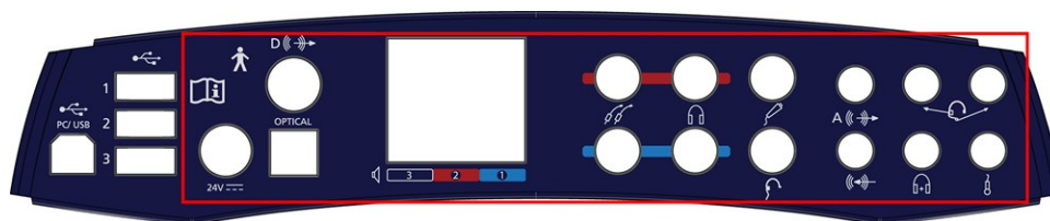
Fig. 1 Sockets with direct connections to patient transducers - Aurical Aud connection panel
