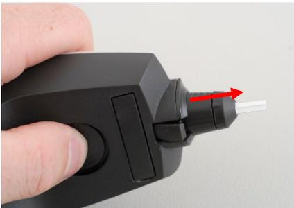
To release the probe or one of the extension cables from the Titan, press the button at the back of the Titan and pull the probe or extension cord out while holding onto the base of the probe or extension cable.
