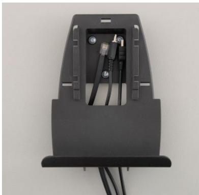
Put the power cable and USB cable behind the retaining plate. Attach these to the cradle before sliding the cradle onto the retaining plate.
