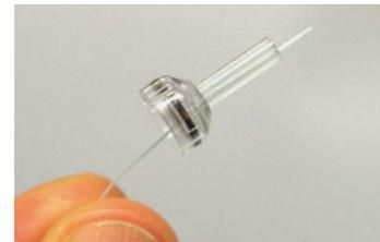
5. Pull the cleaning floss completely through the probe tip tube. Clean each of the tubes as required. Discard floss after use.
