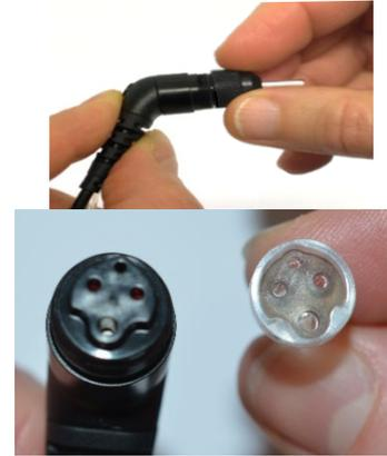
3. For the Clinical Extension Cable probe, to access and clean the larger channel, it is necessary to remove the gasket from inside the probe tip. You can do this using a fine pin. Push the gasket back into place after cleaning.
