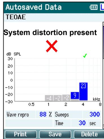
If an error message appears during testing or if one or more of the OAE bands or points has a checkmark (meaning detected), the probe integrity test has failed. This could indicate that:
