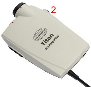
The button (2) on the preamplifier can be used to START or STOP a test.
