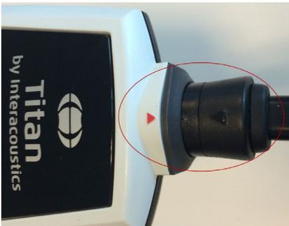
Connect the extension cord or probe to the Titan by lining up the red triangles and pushing the probe or extension cable into the connection plate.
