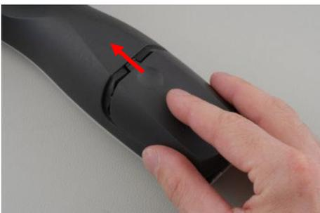
Replace the cover on the Titan and push it upwards to close the battery compartment.
