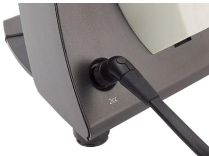
The Titan cradle has a built-in 2cc cavity which can be used for a quick validity check of the probe calibration. You can use the 0.2 ml, 0.5 ml, 2.0 ml and 5.0 ml cylinder cavities for more thorough checks.
